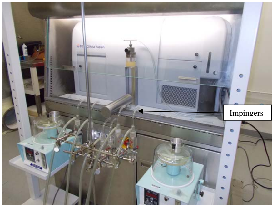
Figure 4: China Standard Personnel Protection Microbiological Test Set Up
