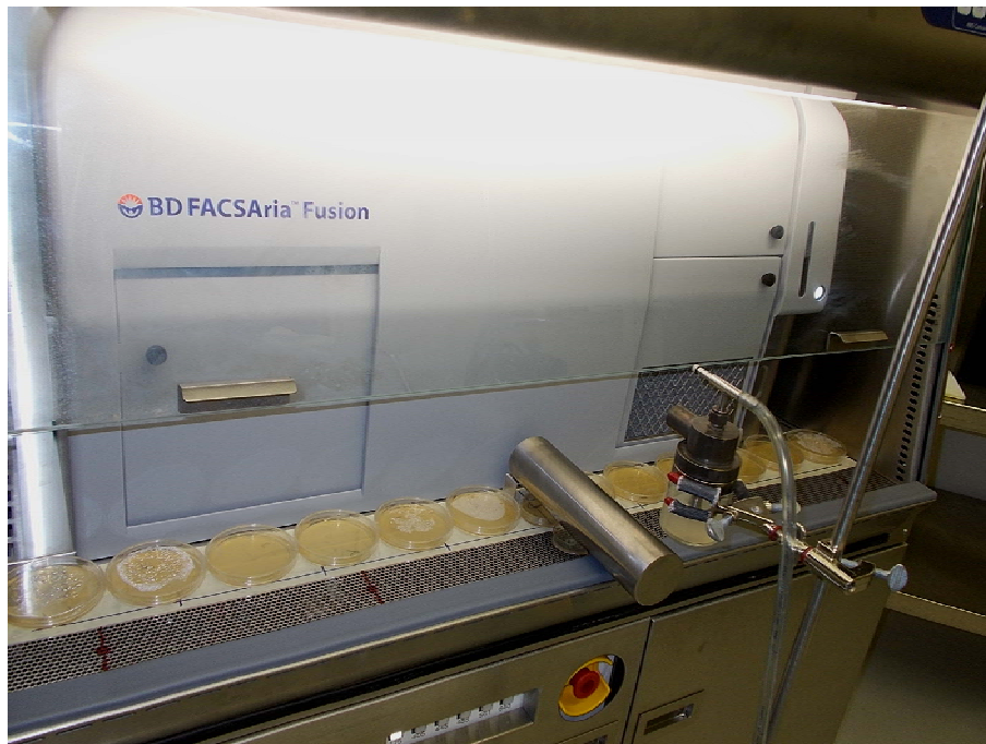
Figure 3: NSF-49 Product Protection Microbiological set-up
