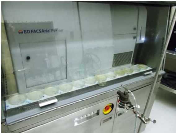
Figure 6&7: “Ready Safe Mode” Product and Personnel Protection Microbiological Tests
