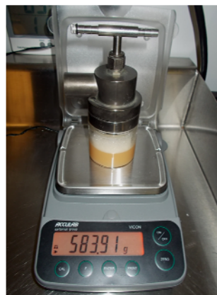
Example of collision nebulizer with 55mls of spore aerosol solution weight before and after each challenge test.
