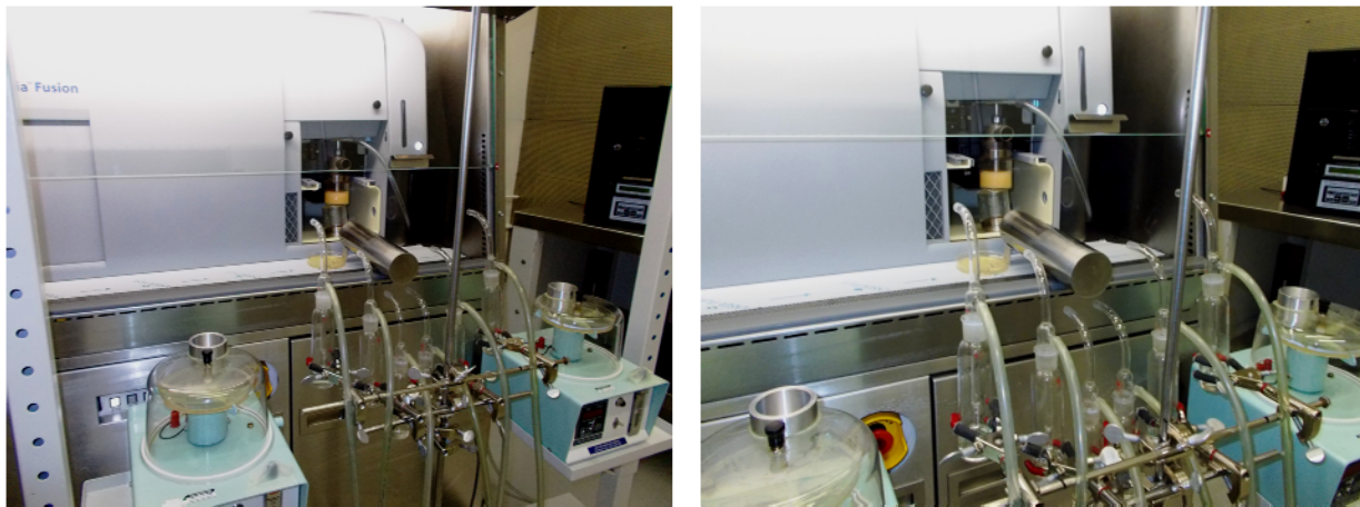
Figure 6: Personnel Protection Microbiological Test at Sort Chamber
