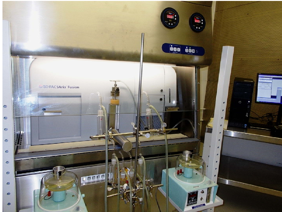
Figure2: NSF-49 Personnel Protection Microbiological Test Set Up
