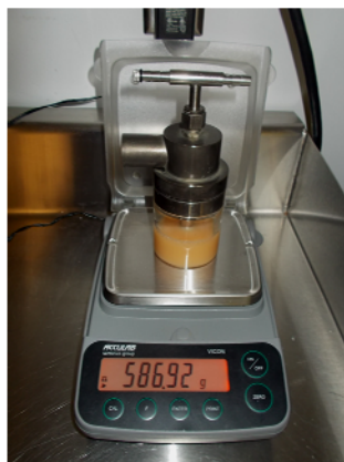
Example of collision nebulizer with 55mls of spore aerosol solution weight before and after each challenge test.
