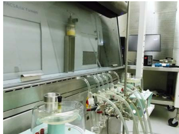
Figure 6&7: “Ready Safe Mode” Product and Personnel Protection Microbiological Tests
