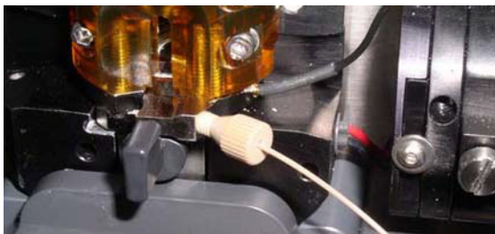
Figure 6-1 Closed-loop nozzle installed in flow cell
