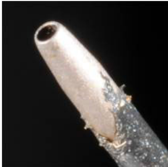
Figure 7-8 Probe with badly worn coating
