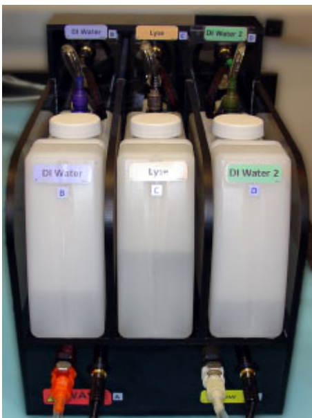
Figure 2-6 Fluidics tower (left) and waste tank (right)
