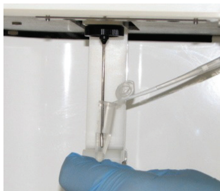
Figure 10. Continuous-flow addition of test compounds with the BD Accuri C6.
