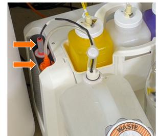
2. Unscrew the disposable waste cap (large cap) and the attached waste trap from the tank. Place the assembly on the bench with the label side up.
